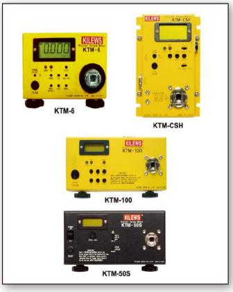
The torque meters are directly produced in Japan, authorized by Kilews Industrial Co., Ltd. by ODM. Each product will be provided with an Adjustment Certificate and one year Warranty in normal using. Take Note! These measuring instruments could not be applied in testing the pneumatic screwdriver products and prohibited in measuring the torque exceeding maximum measuring range of torque meters.
